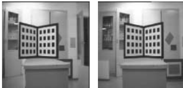
Fig. 7. Pair of images obtained by a moving camera with fixed intrinsic parameters undergoing ground plane motion.
