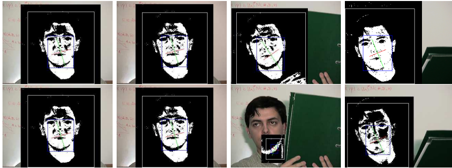
Figure 5: DGW algorithm versus Basic GW without dynamic extension. Basic GW Normalisation with DGW algorithm results are shown in first row. Basic GW without dynamic extension is shown in the second row.
